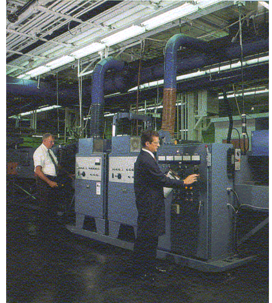
Lion copolymer's technical service laboratory has extrusion and vulcanization capabilities for factory-scale evaluations.
